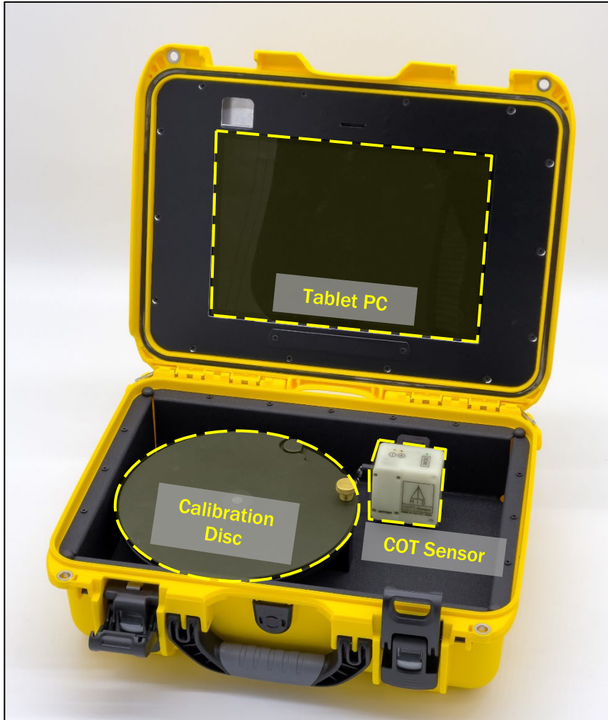
Figure 2 - Changeover Tool (COT) Component Overview
