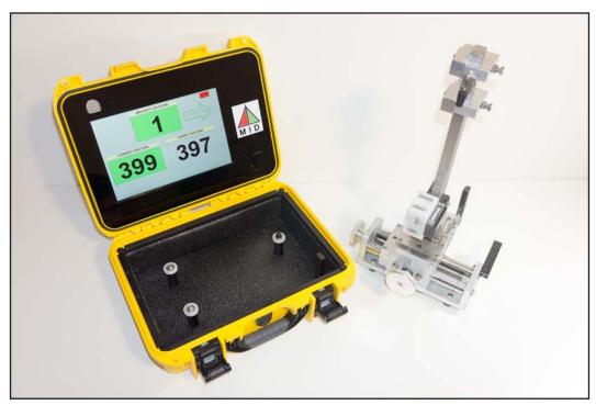
Once the "Zoom" button has been clicked, the screen changes to a more visible layout. The top box (1) is the current bracket number. The bottom left box (399) is the current sensors cable length. The bottom right (397) is the target cable length. The current bracket location adjustment is in position.
