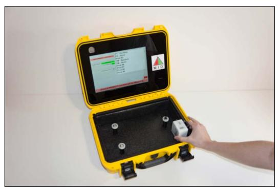
When calibration has been successfully completed, the message banner will instruct the operator to remove the COT sensor from the calibration bracket.
