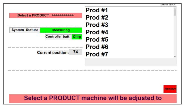
Once the COT sensor is removed from the calibration bracket, the operator is provided with a list of products. The operator should select the desired product adjustment.
