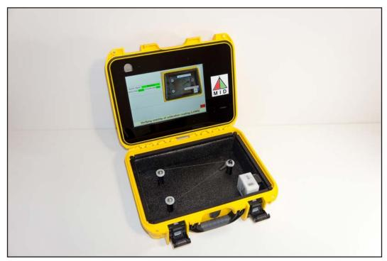
When the sensor ring has been hooked to the long calibration post, the banner indicates that the operator should wait.
