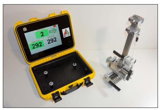
Once cable length is at the target length (or within tolerance), the current cable length box will change from a light red to green. Once the bracket location has been marked as complete, an arrow will indicate to move to the next bracket location.
