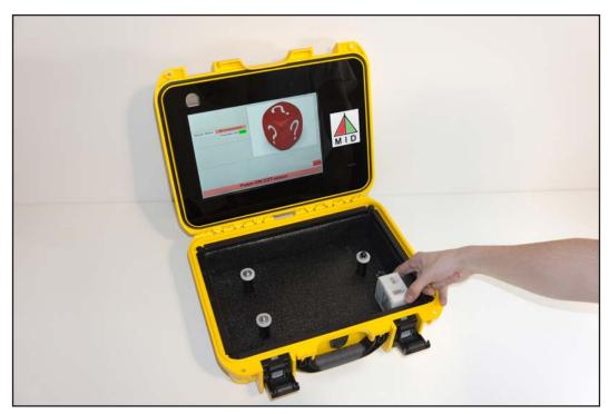
The operator powers on the COT sensor using the button located on the COT sensor. The operator should wait for the COT controller to show that there is communication between the COT controller and sensor.
