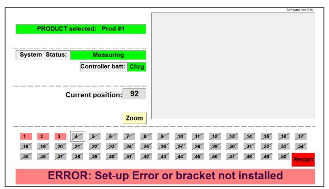
If an error message shows up during the bracket verification, this means that the selected product and machine are not setup for each other. No configurations of that product are present for that machine. This can be changed by the admin in the COT\_CONFIG program.
