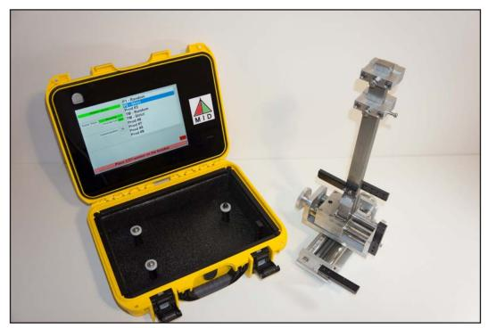
The operator has selected "P2 - Strict" for this demo and is placing the sensor on a bracket located on the machine. The "P2 - Strict" product adjustment will follow a strict ascending bracket adjustment order (1, 2, 3...).
