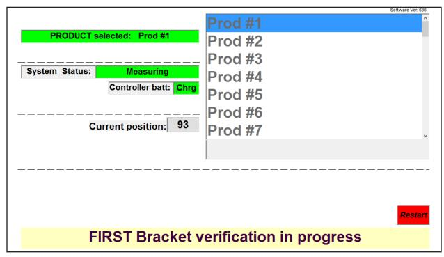
When the COT sensor has been placed on one of the desired machine's brackets, the Changeover Tool will begin the machine verification. At this point, the product selection is locked. Clicking the "Restart" button in the bottom right corner will bring the operator back to the product selection menu.
