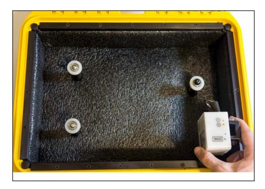
When removing the COT sensor from the calibration bracket, make sure the ring is not attached to a post. Maintain a firm grip on the sensor, and remove the sensor from the calibration bracket.
