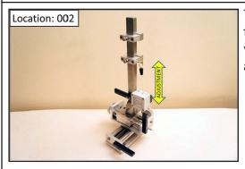
The picture of the current changeover location is shown when the COT sensor is placed on a bracket. This image conatins visual guides for a bracket location such as hook points and adjustment locations.
