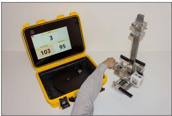
Using the "ZOOM" mode, the user is presented with data pertaining to the current bracket location. This mode can be activated/deactivated at any time during a machine changeover.
