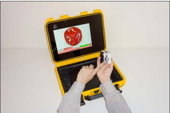
The text banner instructs the user to power on the COT sensor. Remove the sensor from the calibration bracket and power on using the push button located on the front of the sensor. Return the COT sensor to the calibration after it has been powered on.
