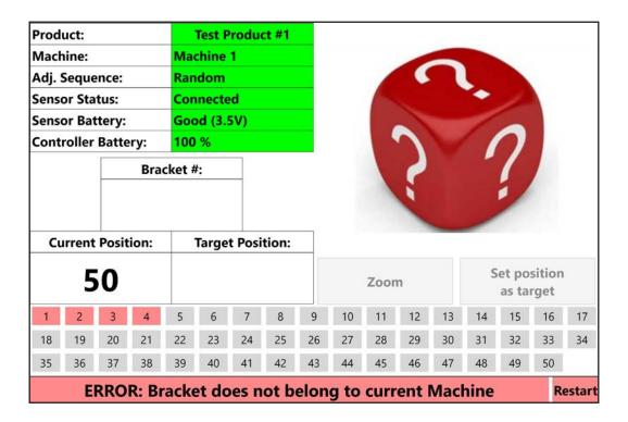
If an error message shows up during the bracket verification, this means that the selected product and machine are not setup properly. The operator should note the error and report it to the system administrator.
