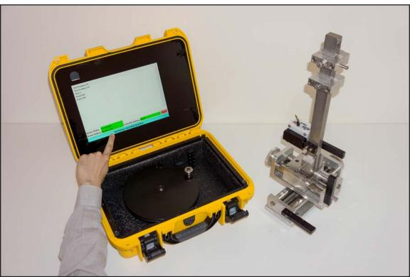
Once the COT sensor has been seated on the first machine bracket, the software will verify the machine bracket number.
