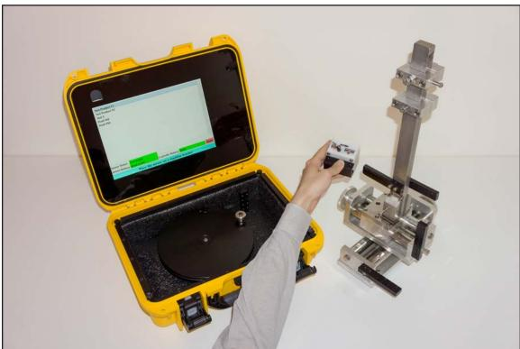
The COT sensor should then be placed on the first bracket located on the machine which is to be adjusted.
