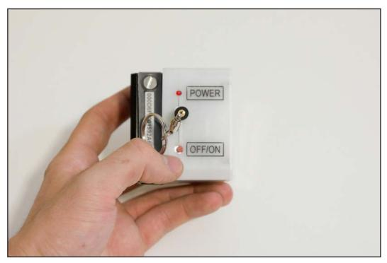
**Step 1**To power on the sensor, press and release the OFF/ON button.
