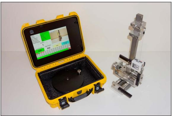
Once the COT sensor has been placed on the next bracket location, hook the ring to the adjustment hook point. Again, verify that the "CURRENT POSITION" value matches the "TARGET POSITION" value. Perform necessary adjustments to satisfy the "IN POSITION" criteria.
