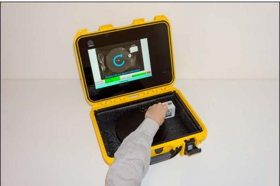
Once the long calibration has been verified, the user will be instructed to rotate the calibration disc CLOCKWISE until the short hard stop is reached. HOLD the disc at the short hard stop.
