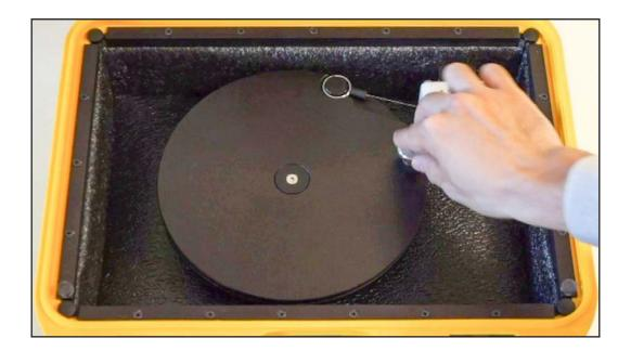
Continue to hold the calibration disc at the hard stop until the software message banner confirms that the long calibration has been completed.
