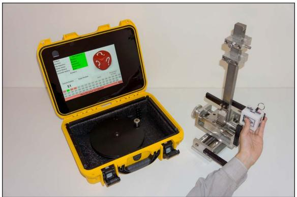
After the bracket location adjustment has been successfully completed, unhook the COT sensor ring from the hook point and remove the COT sensor from the bracket location. Proceed to the next bracket location to continue machine adjustment guidance.
