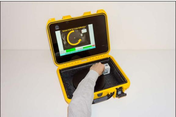
Hook the sensor ring to the calibration disc and rotate the disc COUNTERCLOCKWISE until the hardstop is reached. HOLD the disc at the hard stop until the next instruction is displayed in the text banner.
