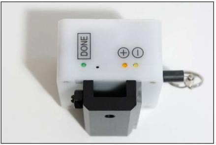
The COT sensor has three LED indicators. These LED indicators consist of a "minus", a "plus" and a "done" LED.
