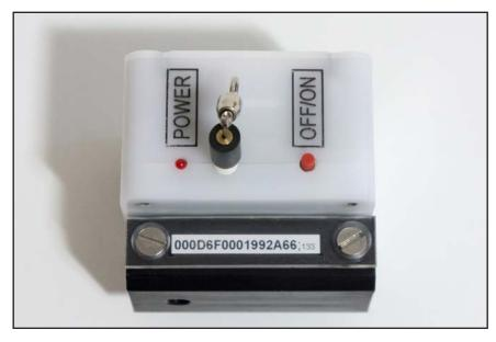
The COT sensor has a "power" LED indicator. This indicator is lit when the COT sensor is powered on.
