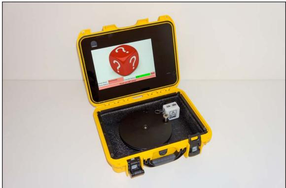
Once the COT Controller has booted, the operator is asked if the machine is ready for changeover. Clicking *"YES"*, the user advances to the sensor calibration screen. The instruction banner instructs the user to power on the COT sensor.
