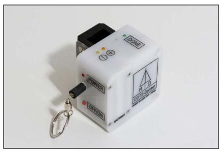
The COT sensor has 4 LED indicators to provide guidance to the operator. This allows for adjustments to be performed without the visual aid of the COT Tablet PC screen.
