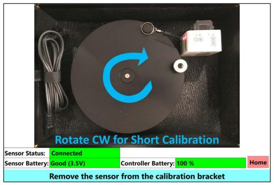
The system will verify the short calibration distance. Once complete, the user will be instructed to "Remove the sensor from the calibration bracket" via the message banner. Remove the COT sensor from the calibration bracket.
