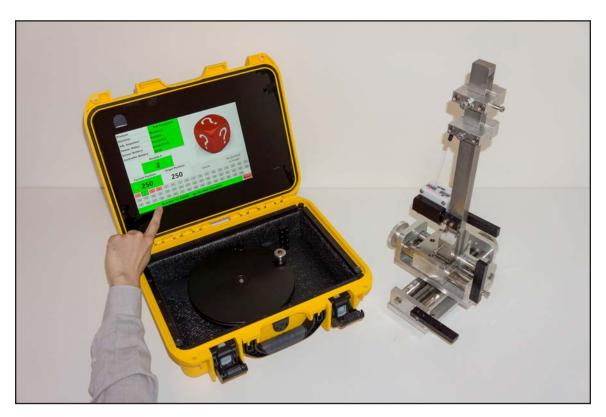
The "Current Positon" must match the "Target Positon" value in order for this bracket location to be considered "IN POSITION". Once "IN POSITION" has been satisfied for 5 seconds, the COT software will confirm the bracket location has been successfully adjusted.
