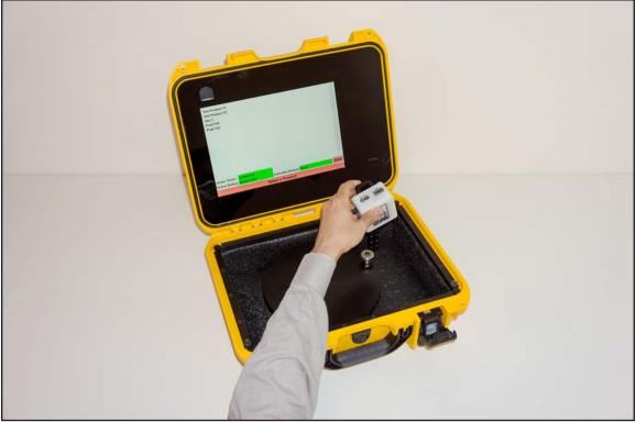
At the compeletion of the COT sensor calibration, the text banner instructs the user to remove the COT sensor from the calibration bracket.
