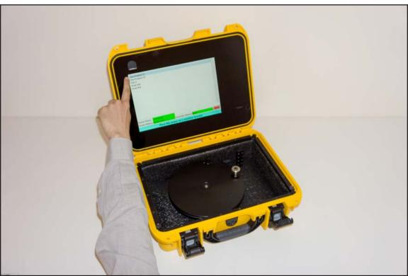
Removing the COT sensor from the calibration bracket will advance the COT software to the product selection menu. On this menu, the user will select the product to which the machine will be adjusted.
